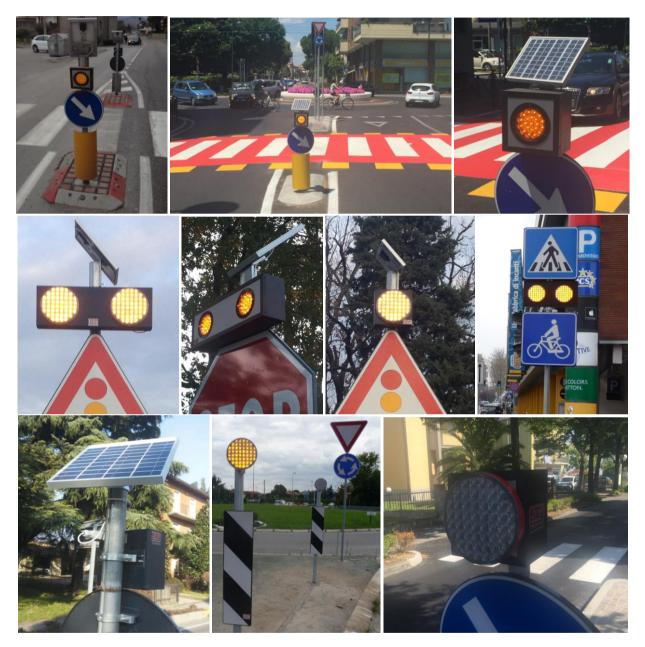
SolarFlash LED flashing lights have LED projectors with a diameter of 100/200mm, complying with standard UNI EN 12352 cl.2H/8H, inserted in single (200x200mm) or double (600x200mm) galvanised aluminium cases.
